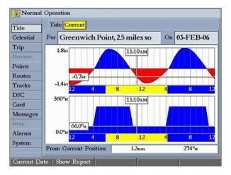
The Current sub tab contains two charts, one for speed and one for direction.
